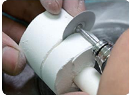
Separate the investment ring using a separating disk and break predetermined breaking point
